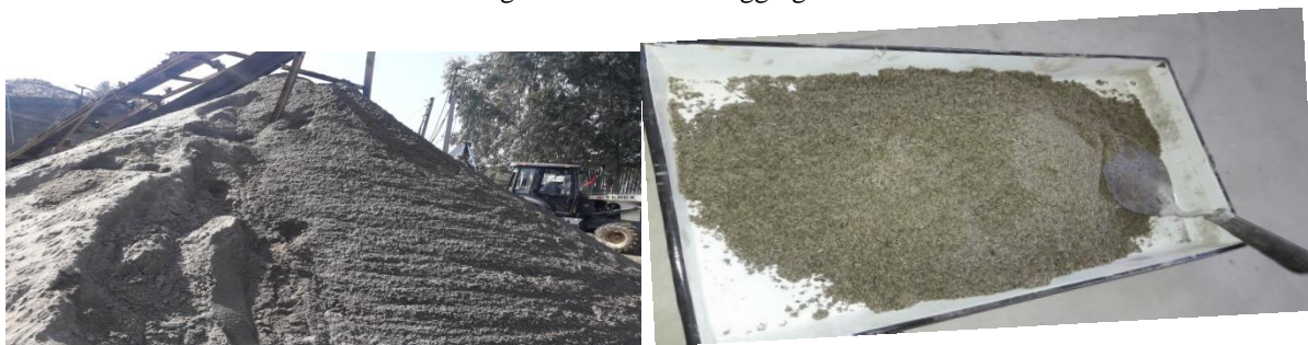
Figure(2) fine Aggregate (sand)
